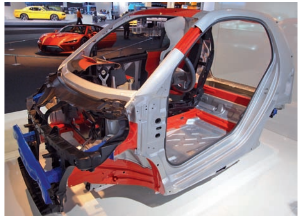
FIGURE 1-7 Safety is another key aspect of the evolution of the modern automobile. As vehicles become smaller and lighter, manufacturers must develop new technologies to keep the passengers and pedestrians safe.
