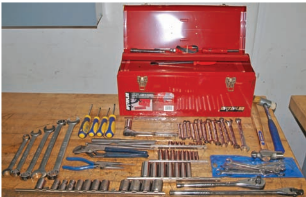
FIGURE 1-9 An example of a starter tool kit, suitable for an entry-level technician.
